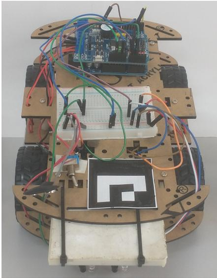
Fig. 3. ArUco Marker placed on the top of the prototype robot.
