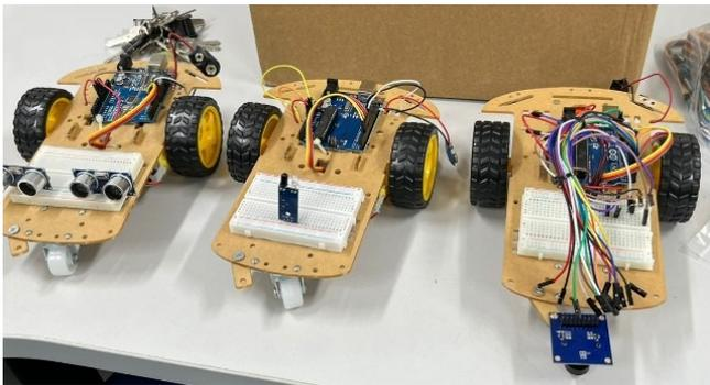
(b) Universal wheel and two wheels connected to a DC motor.
