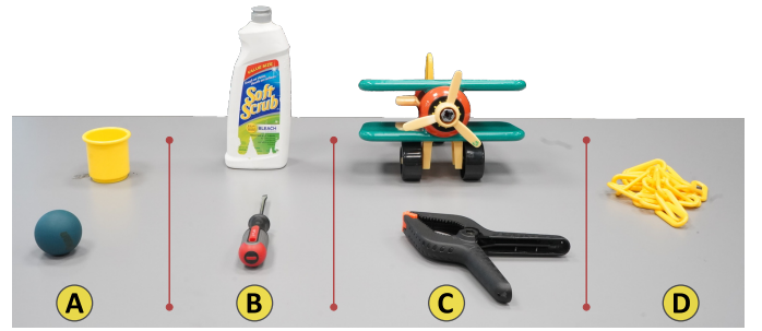
Fig. 2. Selected experiment objects with different complexities. (A) Simple objects: racquetball (YCB ID: 53), yellow cup 19g (ID: 56); (B) moderately complex objects: flat screwdriver (ID: 43), scrub cleanser bottle (ID: 20); (C) complex objects: spring clamp (ID: 46), assembled toy airplane (ID: 67); and (D) deformable object: chain (ID: 61).
