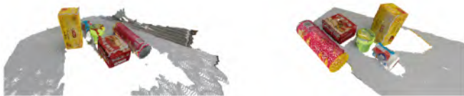
Fig. 8: An example of a labeled scene: the same scene in two view angles. Object models are projected into the scene using the labeled per-scene poses.
