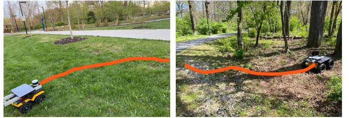
Fig. 1: Trajectories generated by AdaptiveON (ours) when navigating Clearpath Jackal and Husky robots on complex outdoor terrains: Our method ensures stable navigation by reducing vibrations of the Jackal robot on a slope with uneven texture (left); AdaptiveON provides reliable motion control along the trajectories to prevent the Husky from drifting on slippery terrains, including weathered leaves, small rocks, and grass (right).
