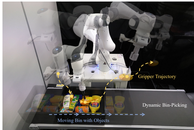
Fig. 1. Dynamic bin-picking: The robot picks up a single object among a cluster of arbitrary objects stacked in a moving bin on a belt conveyor. Our novel framework enables the robot to achieve dynamic bin-picking, ensuring collision-free and adaptive motion. Our method outperforms traditional bin-picking methods in terms of time efficiency, showcasing exceptional effectiveness and reliability in dynamic scenarios.
