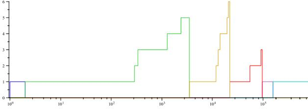
Fig. 11. Simulated number of actual transmitters of first bursts as a function of  $n$  (semilog plot).
