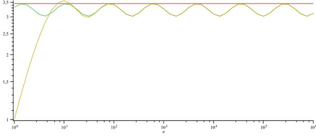
Fig. 4. First burst emitters. Theoretical  $E(C(1, n))$  versus the number of initial contenders  $n$  (semilog plot). Exact theoretical (brown), function  $(\bar{N}^{1/k} - 1) \frac{k}{\log \bar{N}} G(n)$  (green), quantity  $(\bar{N}^{1/k} - 1) \frac{k}{\log \bar{N}} A(k, \bar{N})$  for  $k = 10$  and  $L_N = 3$ .
