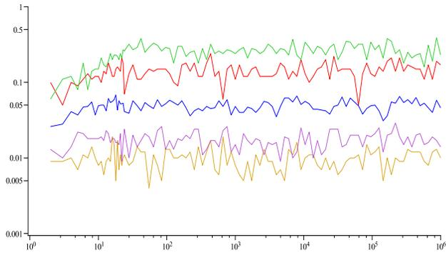
Fig. 16. Mean collision rate in a cognitive WIFI network with an access point as a function of  $\rho$ . From the bottom to the top  $\rho = 0.0$  (brown),  $\rho = 0.1$  (purple)  $\rho = 0.4$  (blue)  $\rho = 0.8$  (red),  $\rho = 1$  (green).
