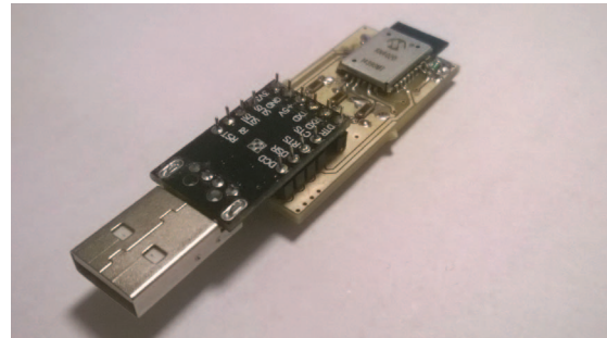
Fig. 6. Picture of the manufactured USB-to-BLE module
