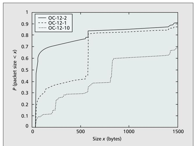
■ Figure 8. Packet size cumulative distribution function.
