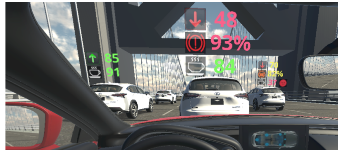
Fig. 7. An example illustration of meta-empowered ADAS: Information is displayed on the ego vehicle's windshield as the augmented reality-based head-up display, which includes neighboring drivers' 1) proficiency scores and their trends, 2) possibilities of certain potential actions (e.g., hard braking and lane change), and 3) current mood score.
