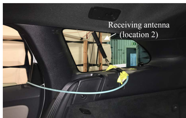
Fig. 2. Receiving antenna at the rear right quarter glass (receiving location 2).
