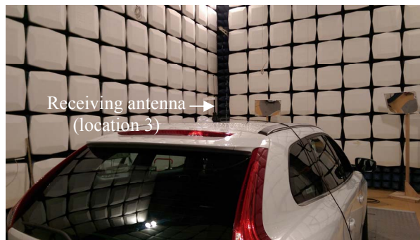
Fig. 3. Receiving antenna on the roof (receiving location 3).
