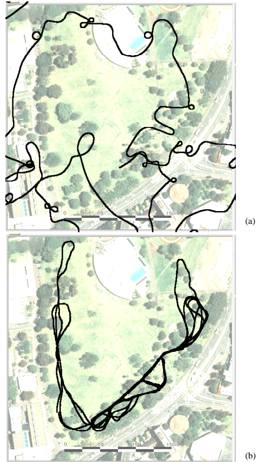
Figure 8: The testing environment: A 350 meters by 350 meters patch in Victoria Park in Sydney. (a) shows integrated path from odometry readings (b) shows the path as the result of SEIF.
