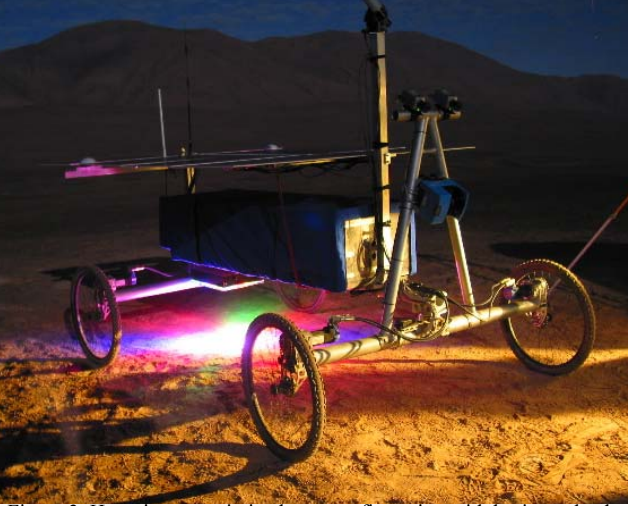
Figure 3. Hyperion rover in its desert configuration with horizontal solar array and underbody fluorescence imager prototype
