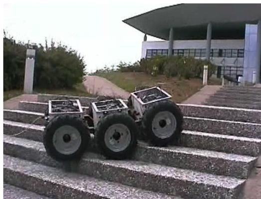
Fig. 1. The RobuRoc mobile robot climbing a stair
