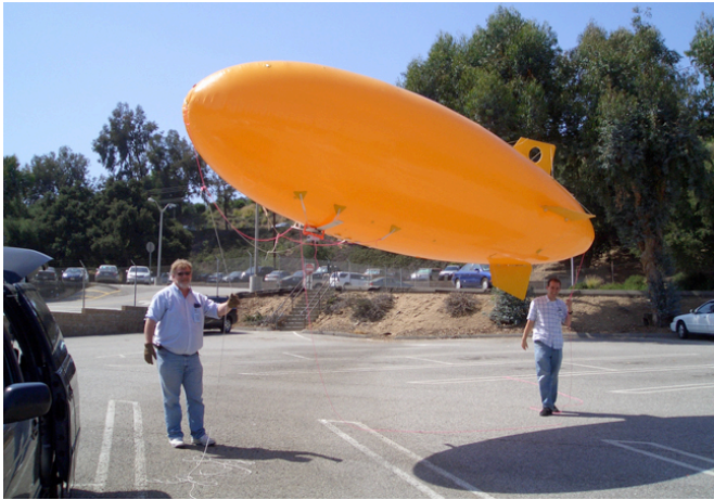
Fig. 9. The TAOSF aerostat observation platform. The aerostat is an unmanned, lighter-than-air (LTA) unpowered blimp on a tether. Helium is used for buoyancy.
