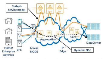
Figure 1: The bold orange line depicts traditional service creation models, following a predefined order of monolithic service elements. The dashed black line depicts dynamic NSC, passing physical and virtual service functions embedded into different network domains.
