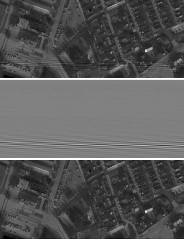
Fig. 5. Simulated data. Top: measured image. Middle: fringe pattern. Bottom: ground truth.
