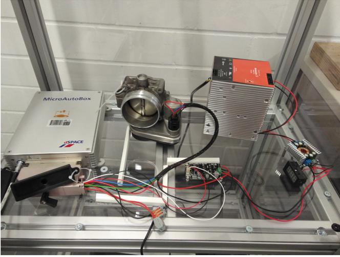
Fig. 5. Experimental setup. The throttle plate is shown in the center. It is controlled via the MicroAutoBox (left).
