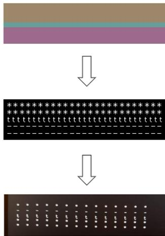
Fig. 4. Image processing result, from the input image to the theoretical output result to the actual output result, the edges of different colors are recognized and converted to ascii code.
