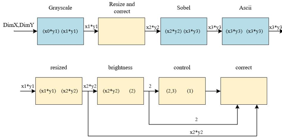
Fig. 3. Image processing task workflow. The blue box represents the processing task, while the yellow box represents the optimization task. The corresponding amount of data will be transferred to the next box upon task completion.
