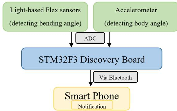
Fig. 7. Physical activity monitor architecture, the sensor transmits data to the STM32 via ADC and finally to the smartphone via Bluetooth.
