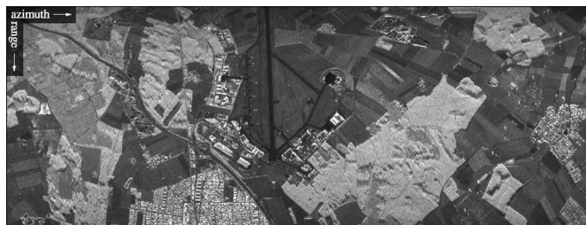
Fig. 7. Reflectivity image of the observed scene. Scene dimensions: 7 \times 2 km (azimuth \times range). Image resolution: 1.3 \times 1.9 m.
