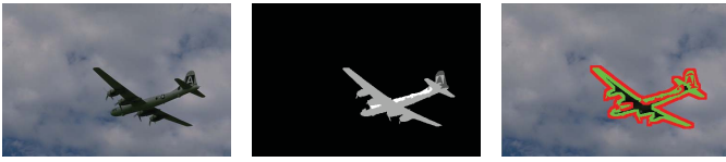
Fig. 9. From left to right. Original image, depth order partition, and f/g labeling on contours. In the depth order partition, white regions are closer to the viewer. In the f/g labels, green pixels belong to the foreground region, the red belong to the ground region.
