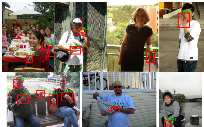
Fig. 9. Examples of high-scoring detection on Oxford hand database(outdoor images). The rotation estimation is illustrated with red arrows.
