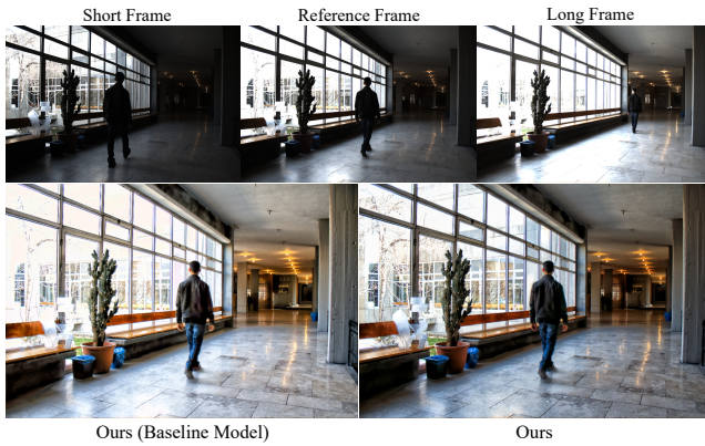
Fig. 6. Qualitative evaluation of our model on a test scene from the Tursun dataset with large foreground motion and severe over/under-exposure. Our exposure uncertainty is able to regulate the contributions of overexposed pixels in the window panes while our max-pooling mechanism restores details which are not visible in the reference frame.
