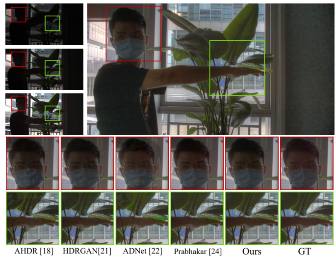
Fig. 13. Qualitative evaluation of our method for an image from the Chen test set. Our method performs well even in low light conditions while other deep learning methods suffer from ghosting and artefacts. Best viewed zoomed in.
