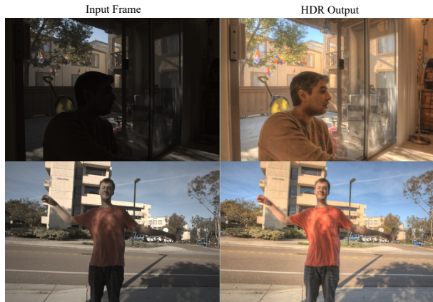
Fig. 16. Qualitative evaluation of our model using just the short frame as input. When the input frame is severely underexposed (top), we see quantization and noise related artefacts. However when the input frame is well exposed (bottom), the output is free of artefacts.
