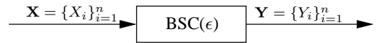
Fig. 2. Section V-A setup: \mathbf{X} is a binary first order Markov process with transition probability p , and \mathbf{Y} is the output of a binary symmetric channel with crossover probability \epsilon corresponding to the input \mathbf{X} .
