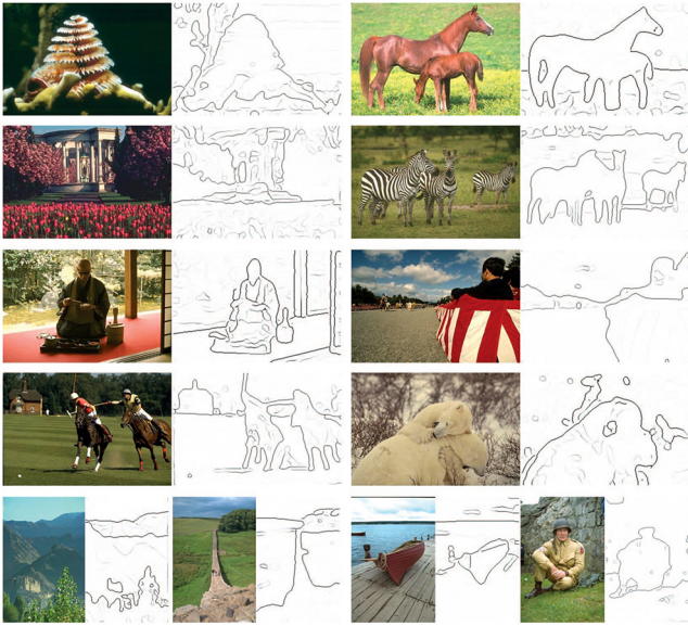
Fig. 13. Boundary detection examples, obtained using a Gb model that uses only the first 3 dimensions of our soft-segmentations as input layers. Note: Color layers were not used here.
