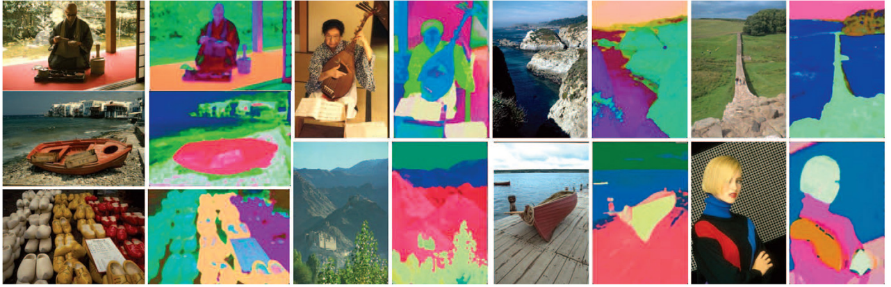
Fig. 7. Soft-segmentation results from our method. The first 3 dimensions of the soft-segmentations are shown on the RGB channels. Computation time for soft-segmentation is \approx 2.5 seconds per 0.15 MP image in MATLAB.
