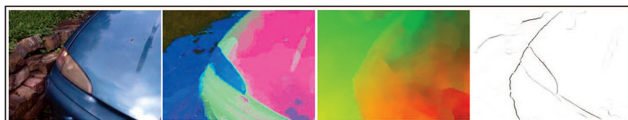
Fig. 1. Gb combines different image interpretation layers (first three columns) to identify boundaries (right column) in a unified formulation. In this example Gb uses color, soft-segmentation, and optical flow.
