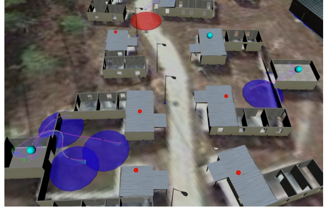
Fig. 1: Persistent Surveillance under Attacks. Unity simulation environment depicting a 5-robot team engaging in a Persistent Surveillance task for monitoring a set of buildings. Some robots are under attack. The attacks can disable the sensing capabilities of the robots, at least temporarily. Each blue disc indicates the field of view of a (non-attacked) robot, while each red disc indicates an attacked robot. In this adversarial environment, the robots must resiliently plan trajectories to (re-)visit all the building landmarks to continue acquiring information despite the attacks.
