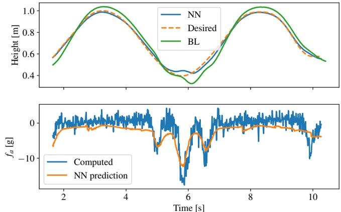
Fig. 9. Generalization to a team of five multirotors. Three small multirotor move in a vertical ring and two large multirotor move in a horizontal ring. The maximum  $z$ -error of a small multirotor in the vertical ring with powerful motors is reduced from 10 cm to 5 cm and  $f_a$  is predicted accurately.
