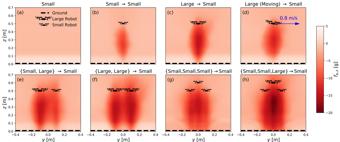
Fig. 5.  $f_{a,z}$  prediction generated by the trained  $\{\rho_{\text{small}}, \rho_{\text{large}}, \phi_{\text{small}}, \phi_{\text{large}}, \phi_{\text{env}}\}$  networks. Each heatmap gives the prediction of  $f_{a,z}$  of a vehicle in different horizontal and vertical (global) positions, and the (global) position of neighboring drones are represented by drone icons. A more detailed explanation is in Sec. VII-C.
