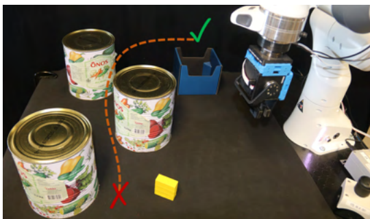
Figure 7. The experimental setup for the case of non-diagonally dominant inertia. A Franka Emika Panda robot mounts an ATI Mini45 force/torque sensor and a QB SoftClaw gripper. The object (■) should be grasped and transported from the initial (X) to the goal (✓) position.
