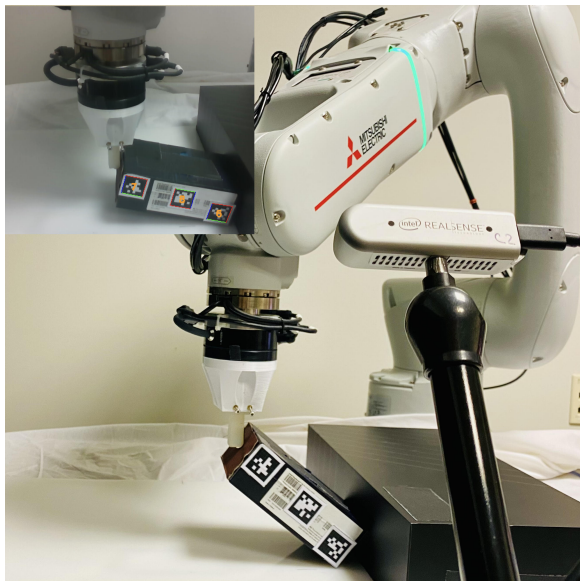
Fig. 22: The vision-based feedback pivoting system which can observe the state in real-time and adapt to recover from disturbances during execution. The inset image shows the tracking of the object using an Apriltag system.
