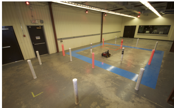
Fig. 5: Setup for Experiment 1. A wheeled robot drives around 17 cylindrical landmarks (2 are not visible in this photo) in an indoor environment. It logs wheel odometry and measures the range to its surrounding landmarks using a laser rangefinder. The landmarks for testing are highlighted in red.
