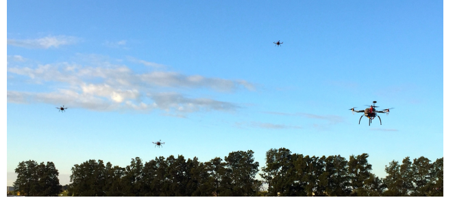
Fig. 1: Mobile wireless infrastructure on demand. A team of UAVs acting as network providers continuously reconfigure their positions and communication routes, provisioning task users with their required quality of service in terms of wireless connectivity.
