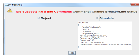
Fig. 2: An alert message sent from the RTU to the CC.
