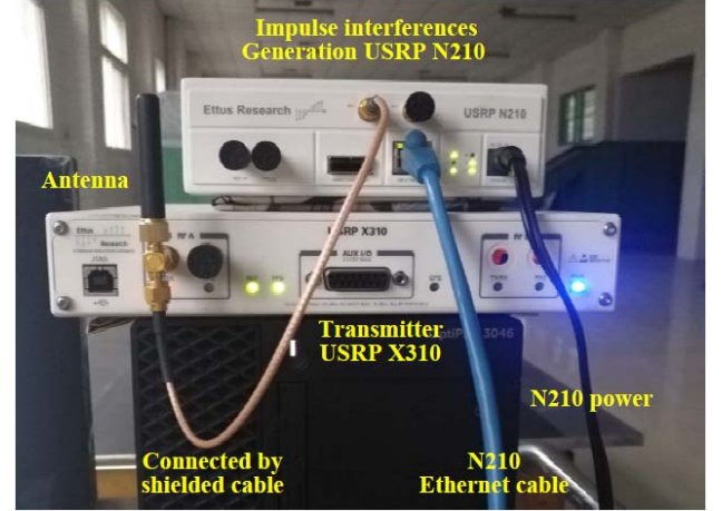
Fig. 7. Connection of impulse interference generator USRP N210 to transmitter USRP X310.
