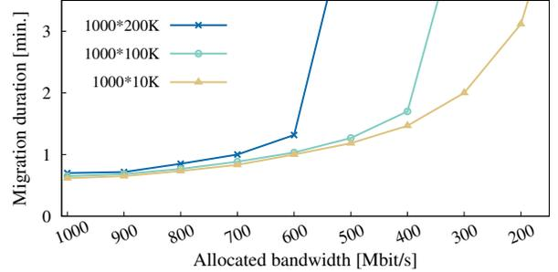
Figure 4. Duration of a live-migration between 2 KVM hypervisors depending on the allocated bandwidth and the parameters used by the command *stress* to generate dirty pages. *1000\*10K* indicates the VM runs 1000 concurrent threads that continuously allocate and free up 10 KiB of memory each. The VM memory used is set to 4 GiB and the downtime is limited to 30 ms.
