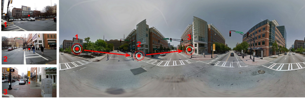
Figure 2. Egocentric FOV localization in outdoor environments. The images on the left are the POV images taken from Glass. The red dot shows the focus-of-attention. The panorama on the right shows the localization (target symbols) and the shifts in the FOV over time (red arrows). Note the change in season and pedestrian traffic between the POV images and the reference image.
