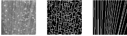
Figure 13: Example of results obtained when a light land scattered with white particles is used for the background. Left side: grey level image (detail); middle: binary image (detail); right side : identified trajectories.
