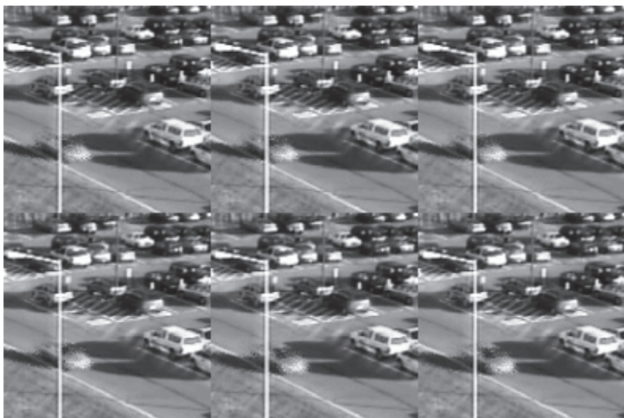
FIG. 7. The reconstruction results of six consecutive frames compressed by our algorithm. The PSNRs for the first row starting from the left are 33.7896, 35.7451, 36.1793, and the PSNRs for the second row starting from the left are 33.7118, 32.6931, 34.7961.
