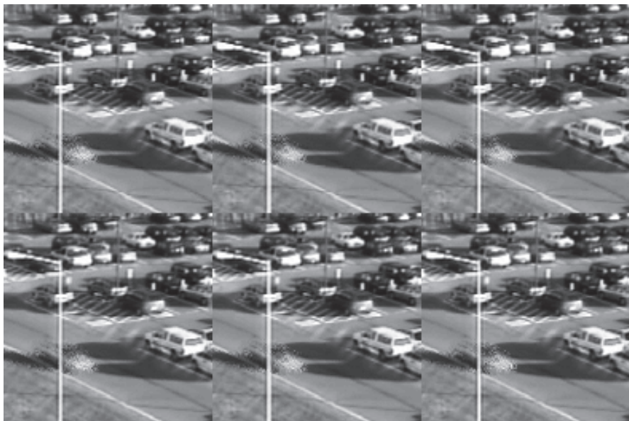
FIG. 8. The reconstruction results of six consecutive frames compressed using a fixed rate, chosen to match the average compression rate of our algorithm. The PSNRs for the first row starting from the left are 32.5228, 33.9217, 34.5397, and the PSNRs for the second row starting from the left are 33.9049, 32.0122, 29.9636.
