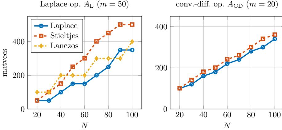
FIGURE 6.9. Number of matrix-vector products for approximating  $A^{1/2}b$ . “Laplace” denotes Algorithm 5.1, “Stieltjes” is `funm_quad` for  $A^{-1/2}c$  with  $c = Ab$ . “Lanczos” denotes the two-pass Lanczos method. The restart length is  $m$ .
