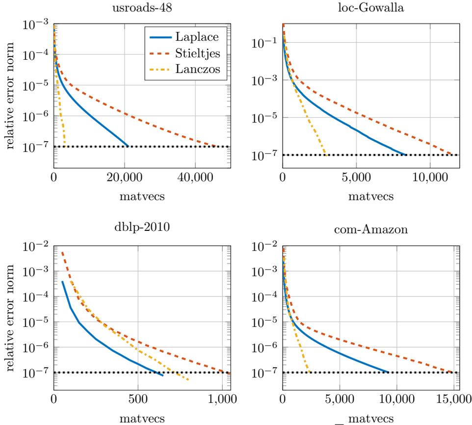
FIGURE 6.6. Convergence curves for approximating  $\exp(-\sqrt{A})b$ . “Laplace” denotes Algorithm 5.1, “Stieltjes” refers to the final error obtained by using `funm_quad` for  $h(A)(Ab)$  in  $\exp(-\sqrt{A})b = (h(A)A + I)b$ . “Lanczos” denotes the two-pass Lanczos method. The restart length is  $m = 50$ .
