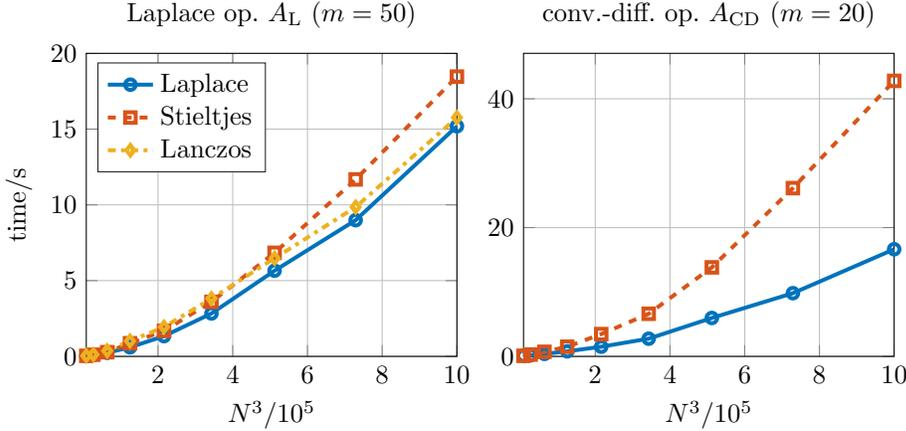
FIGURE 6.4. Execution times when approximating  $A^{-3/2}b$  for varying matrix sizes  $N^3$ . “Laplace” denotes Algorithm 5.1, “Stieltjes” is the combination of `funm_quad` with CG (left) or GMRES (right). “Lanczos” denotes the two-pass Lanczos method. The restart length is  $m$ .
