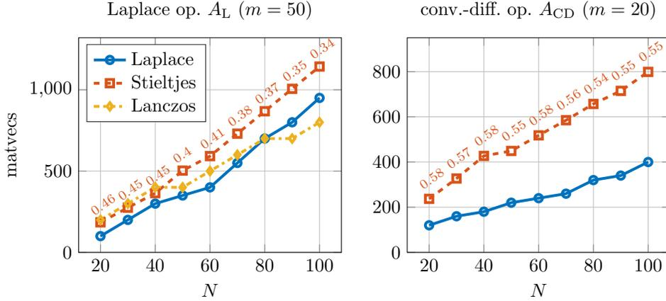
FIGURE 6.1. Number of matrix-vector products for approximating  $A^{-3/2}b$ . “Laplace” denotes Algorithm 5.1, “Stieltjes” is the combination of `funm_quad` with CG (left) or GMRES (right). The small numbers above the dashed line indicate which fraction of the overall number of matrix-vector products was computed in the first phase, i.e., in the CG or GMRES method. “Lanczos” denotes the two-pass Lanczos method. The restart length is  $m$ .
