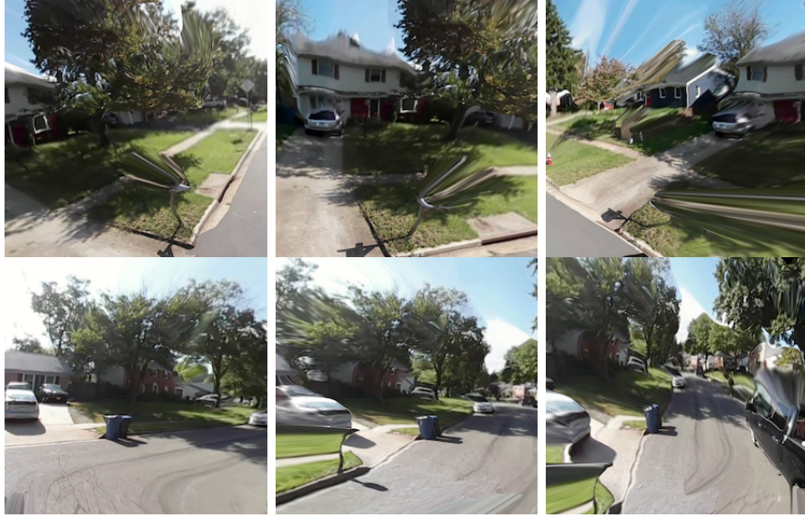
Fig. 13: Examples of new view synthesis using the estimated depth map to create a textured mesh.
