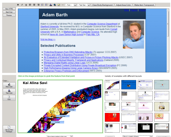
Figure 1 The Adaptive Ideas Web design tool extends a direct-manipulation editing pane ( top ), introducing the ability to browse an adaptively-generated examples gallery ( lower right ), and borrow elements from examples through a preview pane. ( lower left ).
