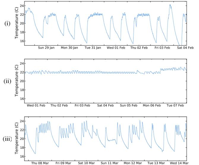
Figure 4. Logger data for three homes, all with set-points of  $22^\circ\text{C}$ , with (i) timed heating periods using an electronic proportional control thermostat, (ii) constant heating using an electronic proportional control thermostat, and (iii) timed heating using a mechanical thermostat.
