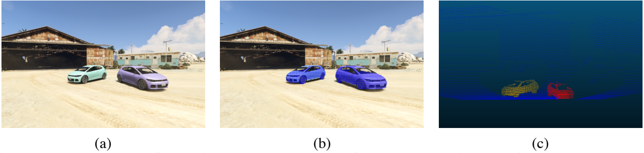
Fig. 1: Sample data extracted from an in-game scene. (a): Image of the scene; (b): Point cloud of car (Blue dots) mapped to image after calibration matches car in image; (c): Extracted point cloud from the same scene.
