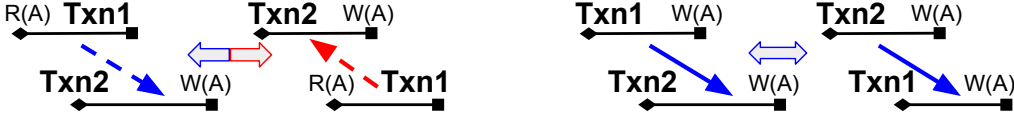
Figure 6: Dependency order preserves between c-rw , anti-rw but not c-ww when switching commit order
