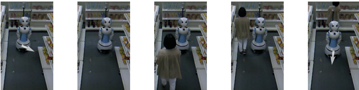
(a) Robot detects the hu- (b) Robot waits. (c) Robot waits. (d) Robot waits. (e) Robot returns to mid- man and steps aside. dle.
