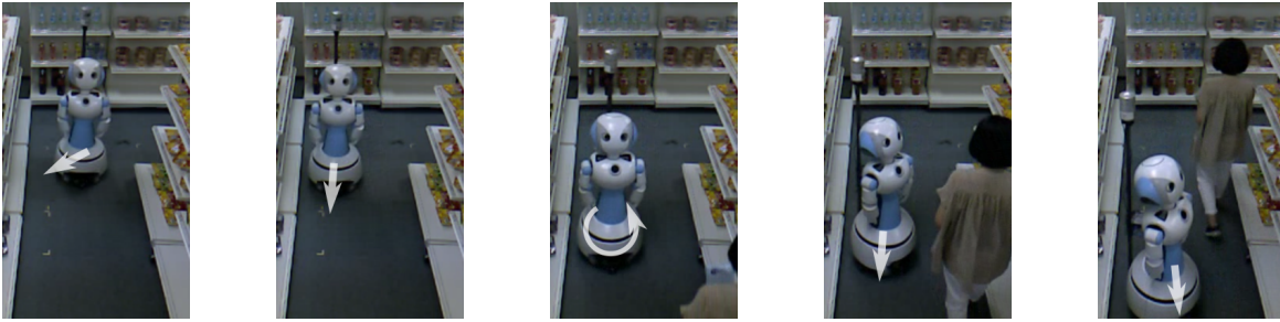
(a) Robot detects the hu- (b) Robot slides forward. (c) Robot rotates its body. (d) Robot keeps moving (e) Robot returns to mid- man and steps aside. forward. dle.
