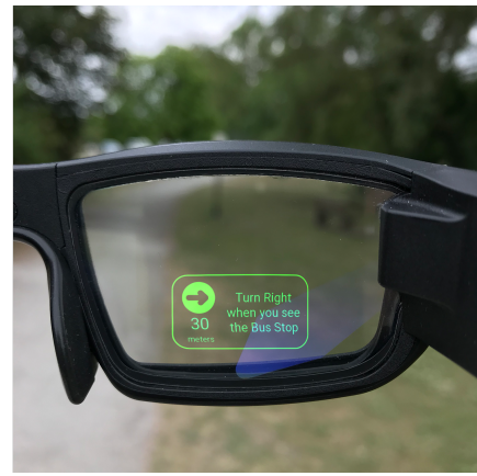
Fig. 2. AR Glasses Application displaying the instruction: "Turn Right when you see the Bus Stop in 30 meters"
