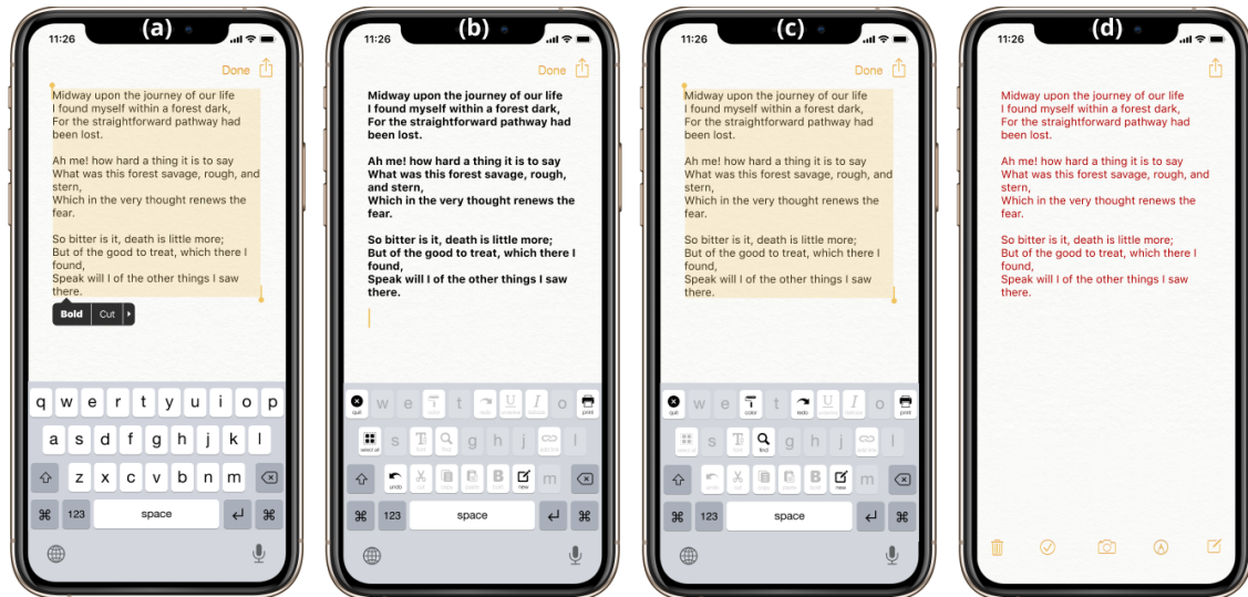
Fig. 3. A demonstration of tasks in a note-taking app that may be done using existing mechanisms or SoftCuts invocations to complete. Participants had to paste text, (a) select all the pasted text, (b) bold the selected text, (c) undo the bold formatting then select all the text again, and finally (d) colour the selected text red. Step (c) and (d) could only be achieved through SoftCuts.
