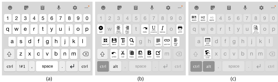
Fig. 26. (a) Example of SoftCuts on an Android soft keyboard with a Ctrl modifier key. (b) Tapping Ctrl once displays the first level of shortcuts (e.g. Ctrl + S for save), and substitutes Ctrl with Alt . (c) Tapping on Alt displays additional shortcuts that are usually triggered with both Ctrl and Alt modifier keys. For this illustration, the Ctrl key is replaced by an Alt key in command selection mode.
