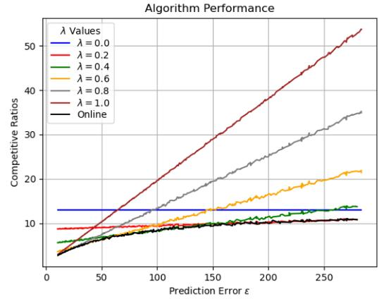
**Figure 1: Competitive ratios of Algorithm 1 and  $\lambda$ -confident control with fixed  $\lambda$ 's for battery-buffered EV charging.**
