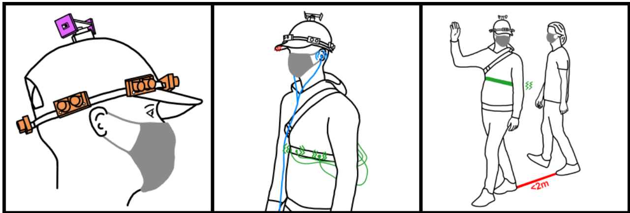
Figure 1: Gapeau augments the sense of distance to others using head-mounted sensors integrated in a hat. We designed three versions of Gapeau with three feedback modalities: visual, vibrotactile and auditory. Our prototype was evaluated in a controlled experiment and during an in-the-wild study.
