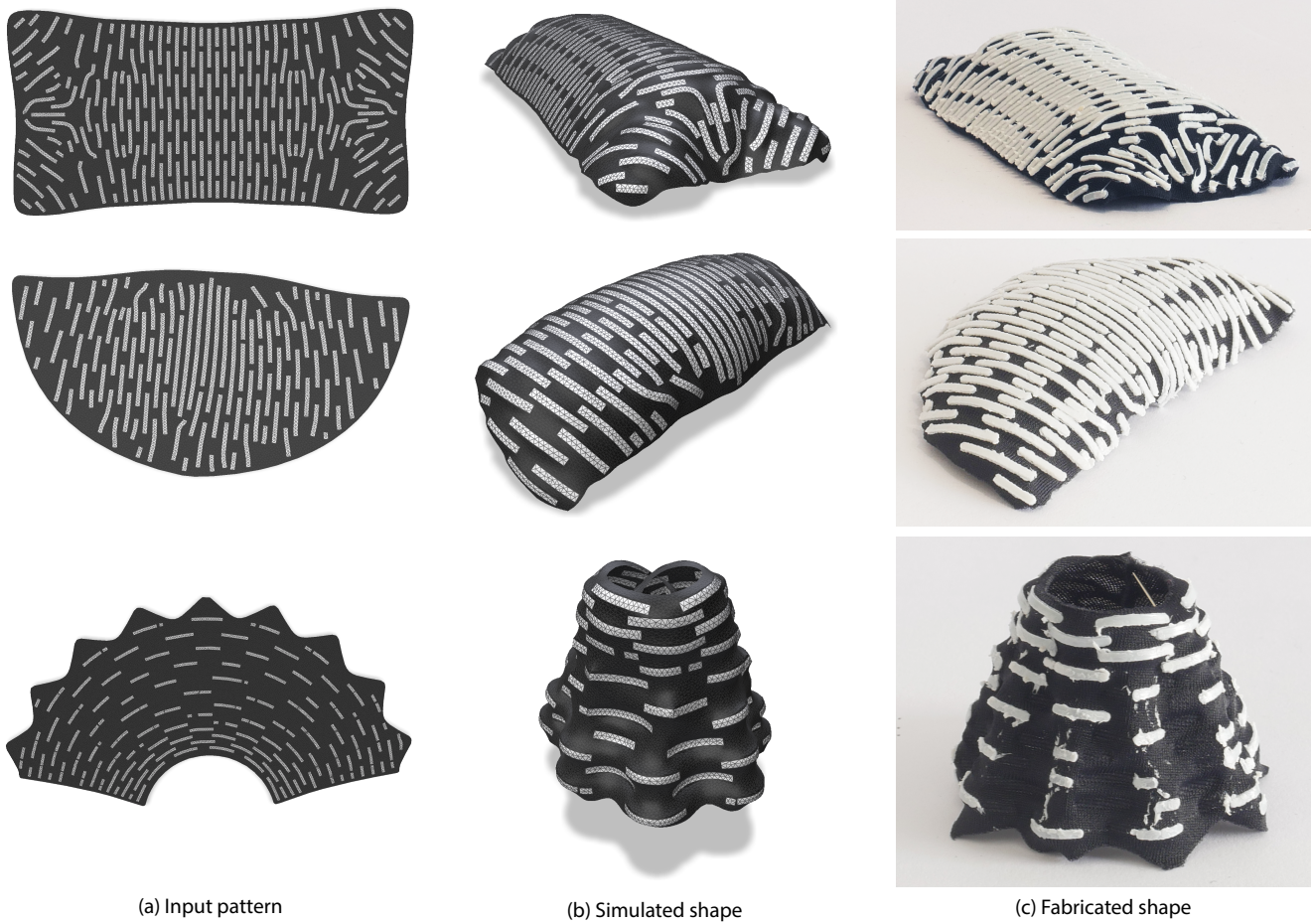
Figure 13: Visual comparison between the results of our simulator (b) and fabricated assemblies (c), using patterns computed with the inverse-design method of Jourdan et al. [2022] (a). The Skirt pattern (bottom row) contains strips printed on the back side of the fabric to produce negative extrinsic curvature.
