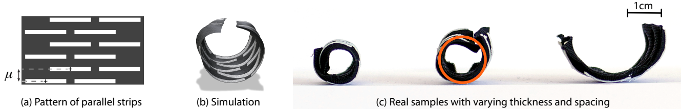
Figure 9: We focused our evaluation on a pattern of parallel plastic strips (a), which rolls as a cylinder when released. Our simulation reproduces well this behavior (b). We fabricated multiple such cylinders by varying the thickness h_p and spacing \mu of the strips (c), and measured their curvature by fitting a circle on their silhouette (c, orange circle).
