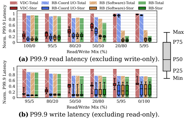
Figure 15. P99.9 latency breakdown. RB is RackBlox. Stor is the storage latency and Total is the end-to-end latency.
