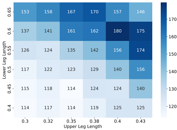
Figure 4: Heatmap illustrating the frequency of selection for each morphology during training on Walker2D. Each cell in the heatmap represents a unique morphology, and the numerical value within the cell indicates the frequency with which that morphology was selected during training. This frequency is computed as the average occurrence across 30 independent training runs.
